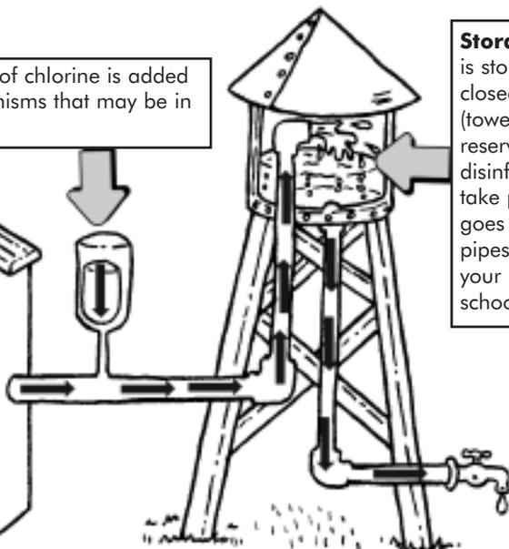
**Storage:** Water is stored in a closed tank (tower) or reservoir so the disinfection can take place. It then goes through pipes and into your home or school.
