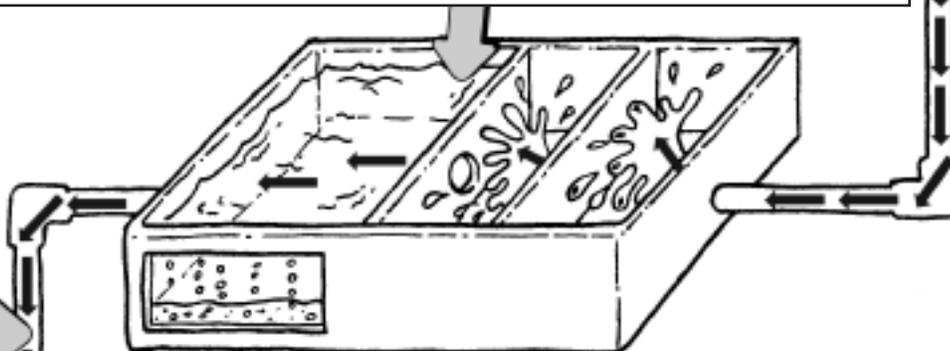
**Sedimentation:** The heavy particles settle to the bottom and the clear water at the top moves on to filtration.
