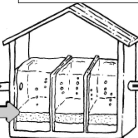
**Filtration:** The water goes through filters, often made of sand, gravel and charcoal that will catch even smaller particles that float in the water.
