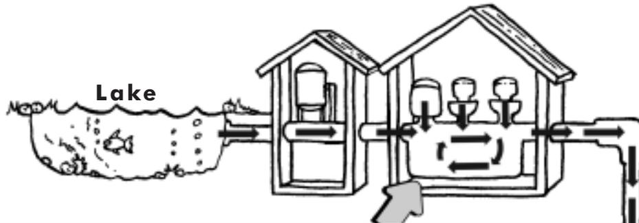
**Coagulation:** Dirty water has many particles floating around in it. Alum and other chemicals are added to the water to form floc that is sticky and attracts the dirt into larger clumps. When they get heavy, they sink to the bottom during sedimentation.
